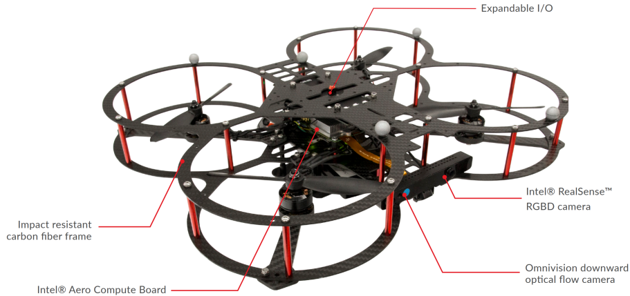
Figure 3.2: Qdrone with components labeled [4]
